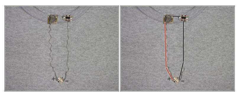
• Continue to make connections with the conductive thread as shown. Be sure to start and finish each stitch with a few finishing knots around each of the circuit board holes.
