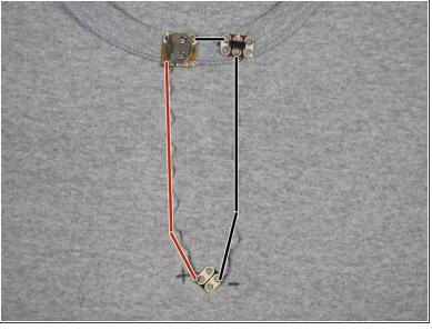
Continue to make connections with the conductive thread as shown. Be sure to start and finish
