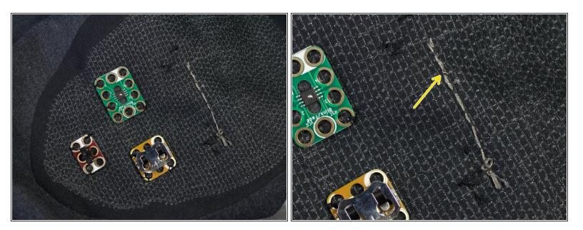
• Turn the shirt inside out. Stitch the thread back along the path. Tie a knot and trim the thread as shown.
