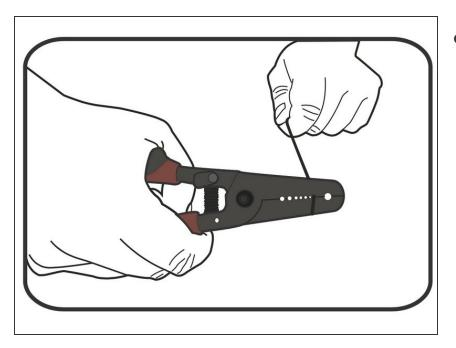
• Strip the ends of all wires, including the Battery Holder.
