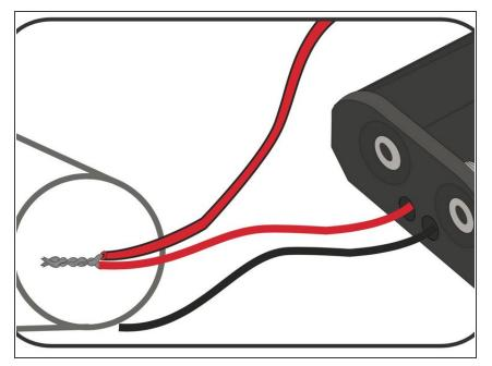
Twist the Red Solar Cell wire together with the Red wire from the Battery holder.
