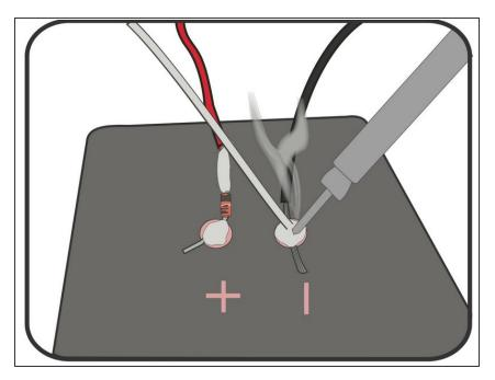
• Solder the loose Black wire to the Negative side of the Solar Cell.
