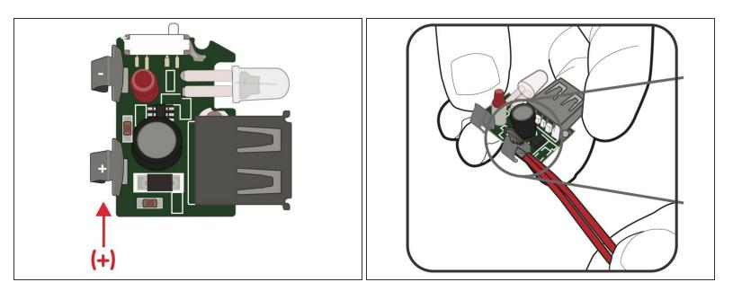
• Solder the Red wires to the Positive terminal on the USB Circuit.
