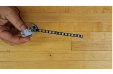
Slide the end of the gate arm on to the shaft of the Servo.
