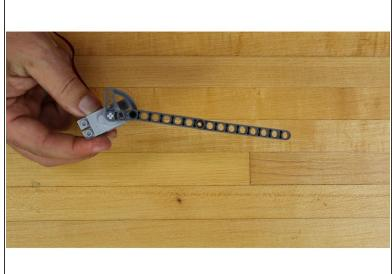
Slide the end of the gate arm onto the shaft of the Servo.
