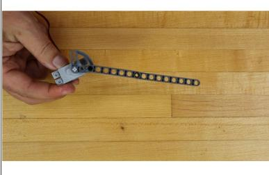
Slide the end of the gate arm on to the shaft of the Servo.
