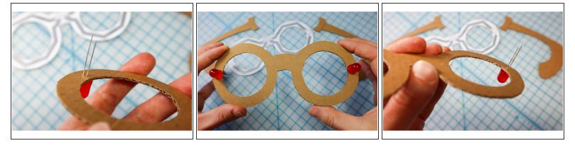
• Push the LEDs through the holes on the frames, with the **Positive** (Long Leg) facing away from the center.
