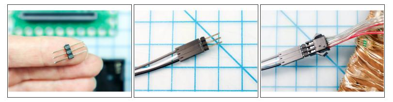
• Plug the jumper wires into the NeoPixel string using three long headers as shown.
