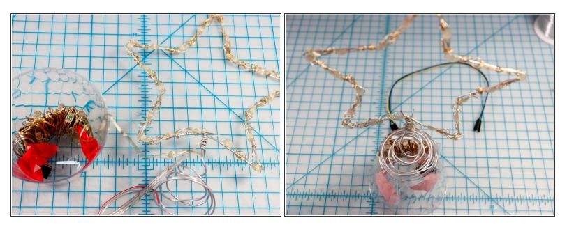
You could trim the NeoPixel strip and remove the unused pixels. However, since they could be unwrapped and reused, hiding the extra pixels inside the cup or in the tree gives you options for later!
