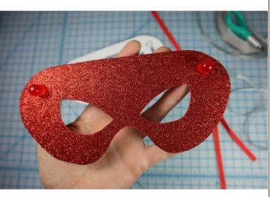
Add a piece of Maker Tape on top of the LED legs as shown.
