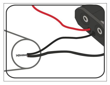
• Twist the Black wire from the Solar Cell together with the Black Wire from the Battery Holder.
