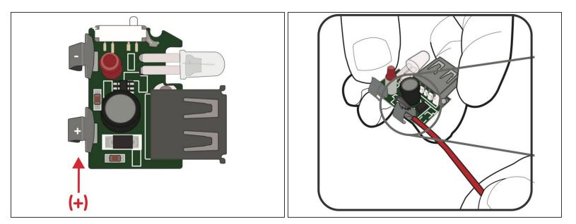
• Solder the Red wire coming off the switch to the Positive terminal on the USB Circuit.
