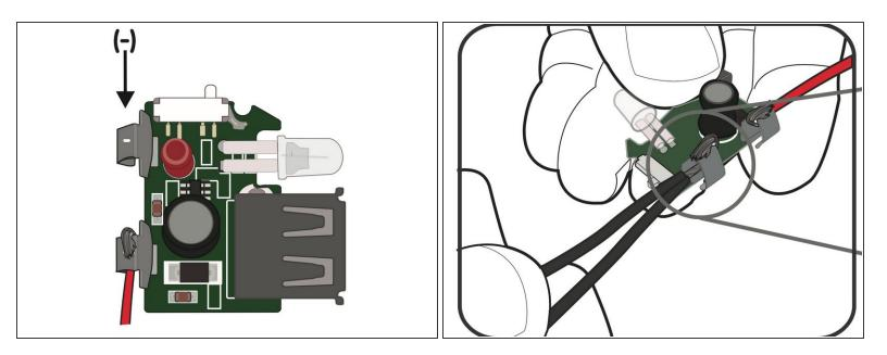
• Solder the two black wires to the Negative terminal on the USB Circuit.
