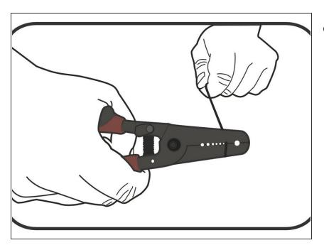
• Strip the ends of all wires. This includes the battery holder.
