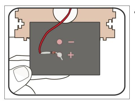
Thread the wire through the "Top" laser cut wood part.
