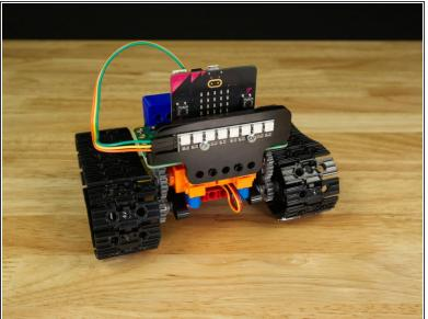
If you have a Bit Board Rover your Addressable RGB LED Strip came attached to a piece of acrylic. This allows it to attach to the front of the Rover using two black pins.
