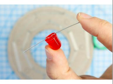
The LEDs have a long positive leg and a short negative leg. Note which is which and bend the LED's legs flat as shown.
