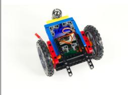
Add the black 11 beams to each set of of pins so the beams stick out the front of the Rover.
