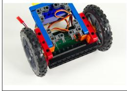
Turn the Rover upside down. We'll add two 90 degree connectors to the blue rear stabilizer beams as show.
