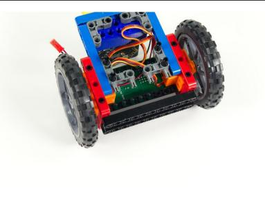
Add four short pins to the 90 degree connectors as shown, two for each connector, in line with the blue beams.
