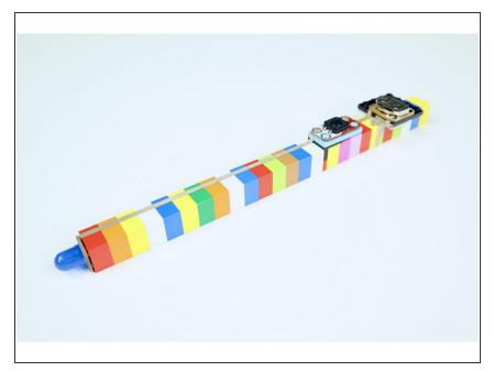
• Here's what your finished wand should look like. Insert a CR2032 battery, hold by the battery holder end and press the pushbutton with your thumb to light the LED at the end!
