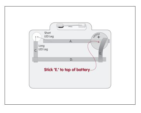
Measure, cut, peel, and stick a piece of Maker Tape down as indicated atop the letter 'E.' and
