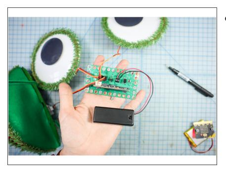
Add a battery pack to the inner tree circuit to make it portable.
