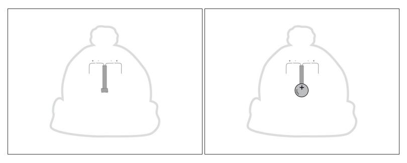
Add a tape loop to the center piece of tape, then stick the battery down to it. (Make sure you stick the negative side of the battery down.)
