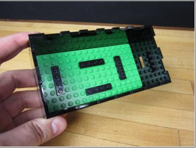
• We threw on some 1x4 plates onto our 8x16 LEGO base plate in order to hold the Robotics Board in place before putting things in our box.
