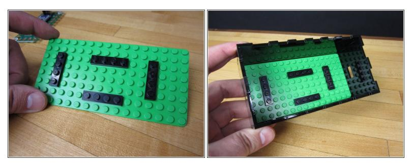
We threw on some 1x4 plates onto our 8x16 LEGO base plate in order to hold the Robotics Board in place before putting things in our box.
