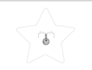
Add a tape loop to the center piece of tape, then stick the battery down to it. (Make sure you stick the negative side of the battery down.)
