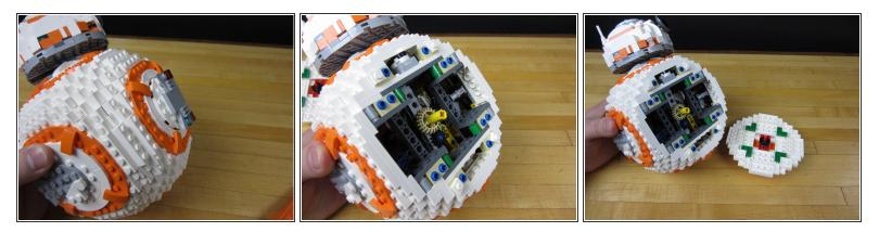
• Using a pry tool, remove the side of BB-8 that controls the head.
