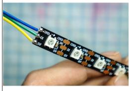
Solder three hookup wires to the +5V, DI, and GND pads on the LED strip.
