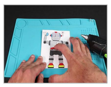
Press on the belt buckle to bring the conductive tape on the back of it into contact with the two small tape chunks on the card below.
