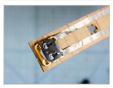
Use a piece of foam mounting tape to place the battery pack at the end of the belt. Double-check that the
