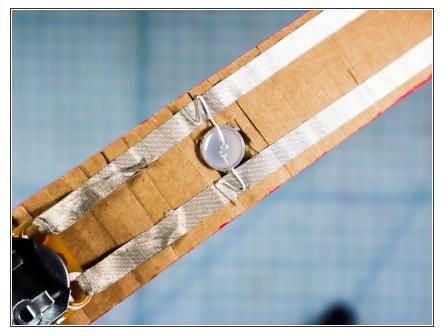
Tuck the LED legs into the belt by folding them back and forth as shown. We've found that this makes a more reliable connection to Maker Tape than cutting the legs.
