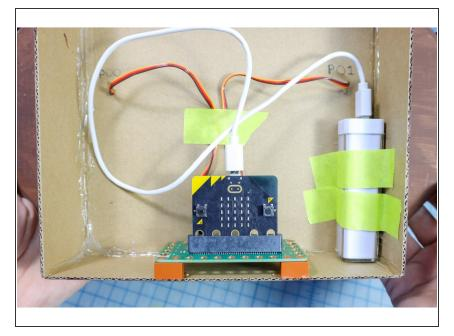
To power the fish, tape a small USB battery pack inside the fish plaque and plug in the micro:bit.
