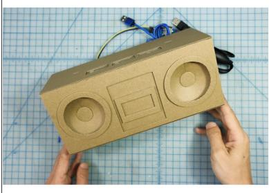
Glue the top of the box to the front and back with Super Glue
