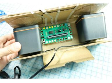
Use foam mounting tape to place the speakers inside the box.
