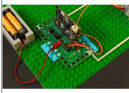
Our circuit consists of a button connected with 1/8" wide Maker Tape to Pin 8 and Ground, and a 270 degree servo plugged into Pin Row 13.
