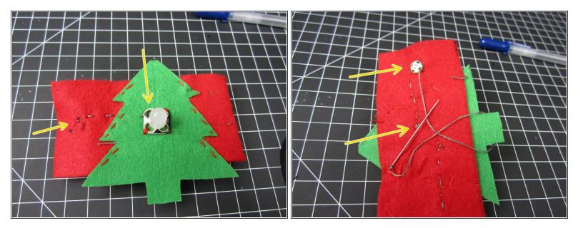
Using Conductive Thread connect one of the white holes on your LED to the other button snap on the opposite side of your fabric.
