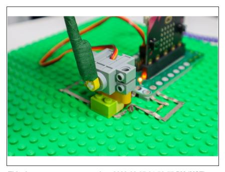
Use LEGO parts to position the servo between the two Light Detecting Resistors.
