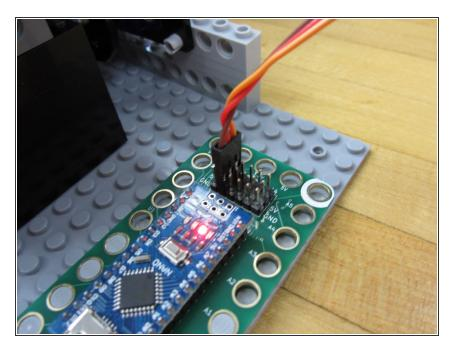
Plug the Servo into the D3 Pin set.
