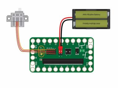
Connect your servo and battery holder to the Bit Board on Pin 1
