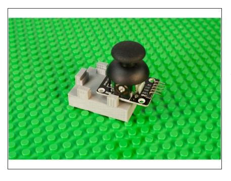
The Thumbstick Sensor slides into the holder and is held in place by friction. If the fit is a bit too tight you
