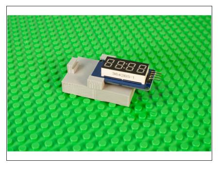
The 7 Segment Display slides into the holder and is held in place by friction. If the fit is a bit too tight you
