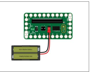
Since we're using a servo a 2 AA Battery Pack is the best way to power our circuit.
