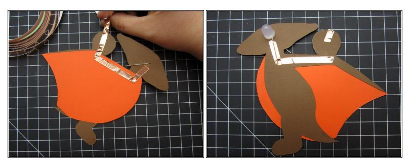
• Run a line of tape from the Positive LED legs back round to the front.
