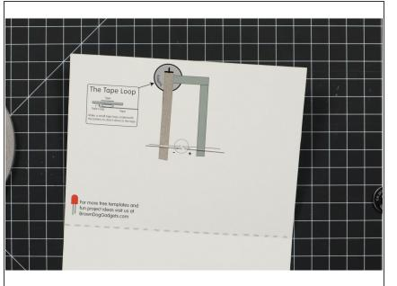
Add a strip of Maker Tape that goes over the negative LED leg and covers about half of the illustration of the battery.
