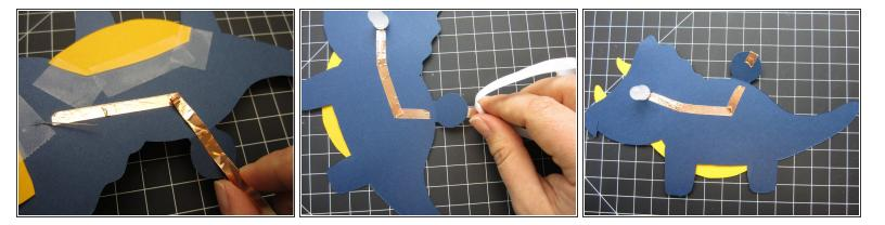
• Run a line of tape from the Positive LED legs back round to the front.
