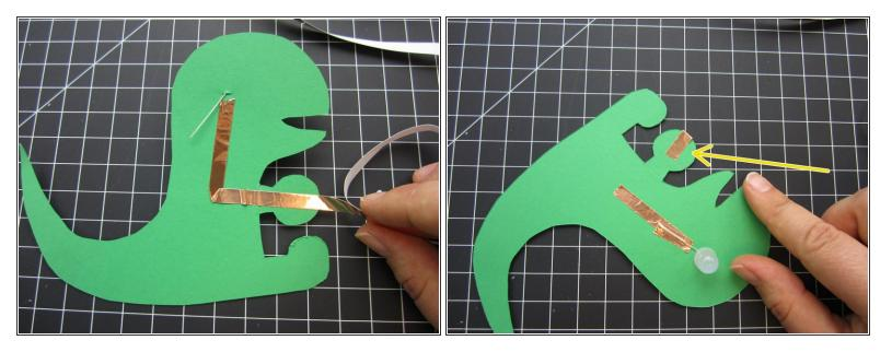
Run a line of tape from the Positive LED legs back round to the front.
