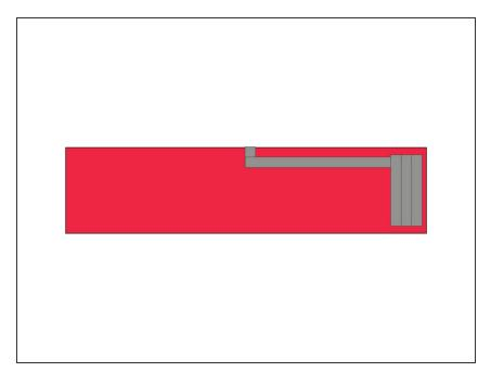
Run a few pieces of Maker Tape over the strip on the back. This part will serve as our "switch" when we connect it to the top with a loop of Maker Tape.
