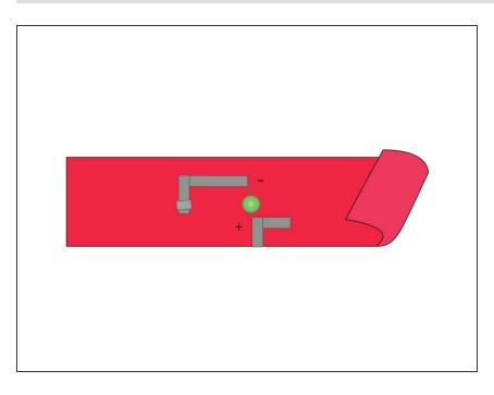
Since Maker Tape is conductive all the way through we can use a loop of tape to hold the battery in place
