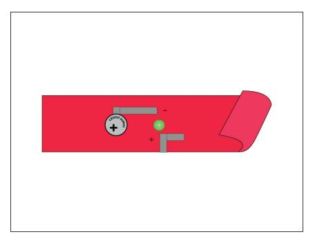
Stick the battery negative side down to the tape loop. You should see the + sign on the battery (which is the positive side) facing up.
