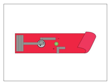
Run a few pieces of Maker Tape over the strip of positive tape that we ran from the top of the battery. This will be our positive connection point for the circuit.
