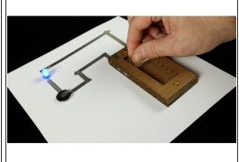
We built a simple circuit using an LED, a battery, and some Maker Tape, and then connected our switch into it. It worked great!
