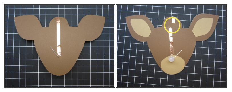
Run lines of tape from the Positive LED legs back round to the front.
