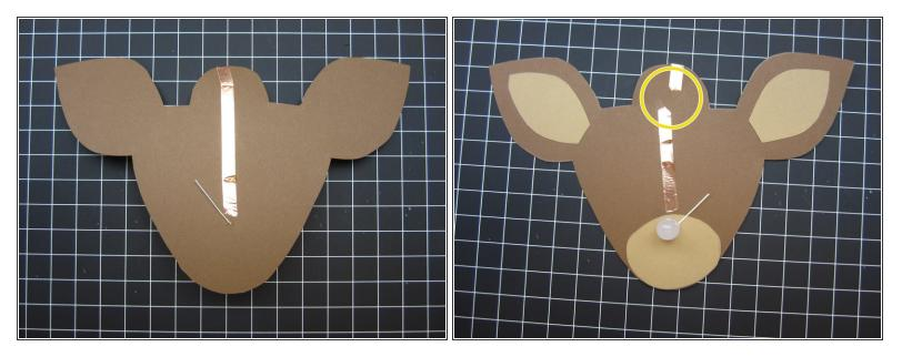
Run lines of tape from the Positive LED legs back round to the front.
