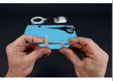
Thread each of your two LEDs through these two sets of two holes. Orient the LEDs so that the long legs go through the holes marked "L" and the short LED legs go through the holes marked "S".
