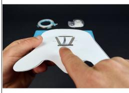
Peel and stick these Maker Tape segments for paths "A,B,C,D". NOTE: "A,B and C" go OVER the LED legs while D simply goes atop paper.
