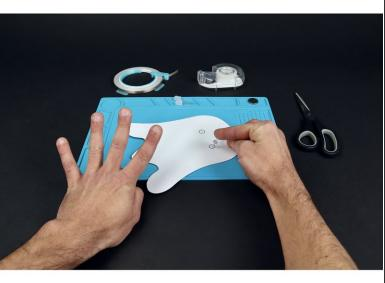
Use a pushpin to poke 4 holes where shown within the two circles that indicate where LEDs will be placed.
