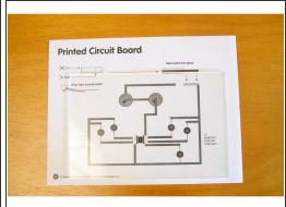
We've provided a PDF that you can print out and place under your clear plastic sheet so you can see your circuit and attach all the components with tape. Make sure your plastic is large enough to fit the entire circuit on.
