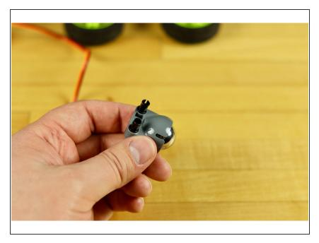
The steel ball and joint allow for a third point of contact with the ground. Use two pegs to stick this on the back of the frame.
