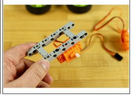
Use some pegs to attach the servo to the frame.
