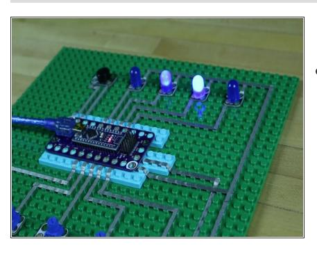
Plug in a USB cable for power and make some noise! As you turn the first four potentiometer dials you will alter each of the four notes. The LEDs will light up as the note plays. Use the fifth potentiometer to adjust the tempo or speed that the notes play.
