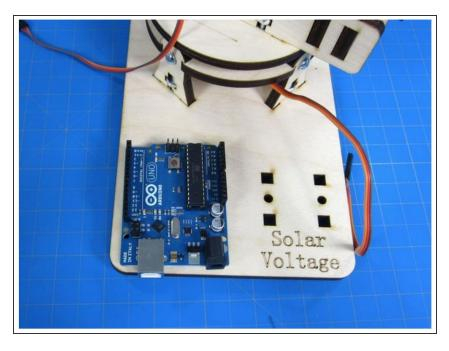
Use two of the M3 screws to screw the Arduino into the base.
