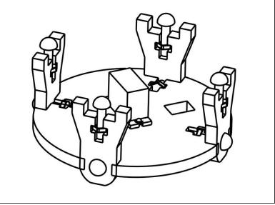
Screw each of the four legs into the center ring.
