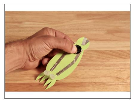
Position your battery so the positive side (marked with a +) faces you and the top edge of the battery itself lines up with the fold below the tab.
