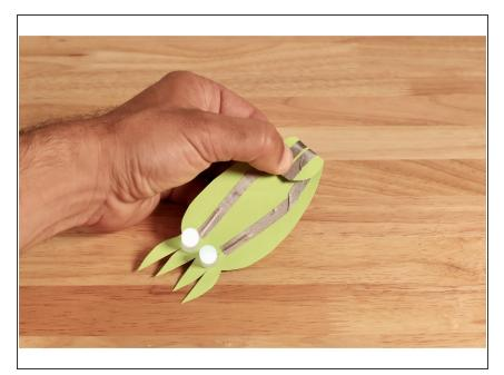
Folding the tab over and pressing it in contact with the top of the battery should cause your LEDs to light up. TIP: If they don't light up, you may have positioned the LED legs incorrectly...flipping the battery over should remedy this mistake.
