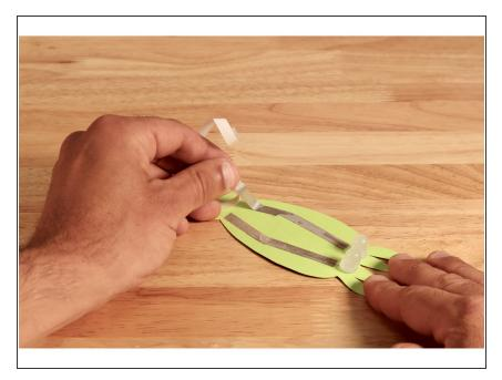
Lay Maker Tape pathways on top of each of the LED legs on the front side so that the two paths are close to one another at the fold line of the tab.
