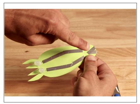
After bringing the tape pathways from the back side to the front, they should end where shown to create a small gap between them and the two paths on the front.
