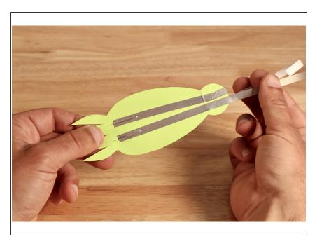
Flip shape over and make two more Maker Tape pathways for each of the legs on the opposite side. Lay the tape PAST the fold, over the tab and to the front side of the tab, leaving a gap between their ends and the ends of the first two paths you made.
