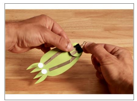
Once the LEDs are lit, secure the battery connection with the binder clip as shown. This should keep the circuit connected to the voltage source for hands-free enjoyment.
